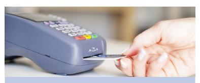
A chip-enabled terminal looks almost identical to the terminals you use today when you swipe your cards. In addition to the magnetic strip reader, chip card terminals have a slot on the front where you will insert and leave your card while your transaction processes.
