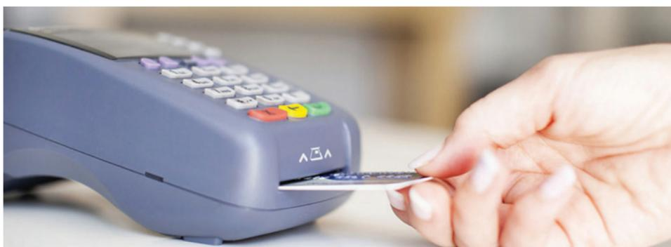
A chip-enabled terminal looks almost identical to the terminals you use today when you swipe your cards. In addition to the magnetic strip reader, chip card terminals have a slot on the front where you will insert and leave your card while your transaction processes.
